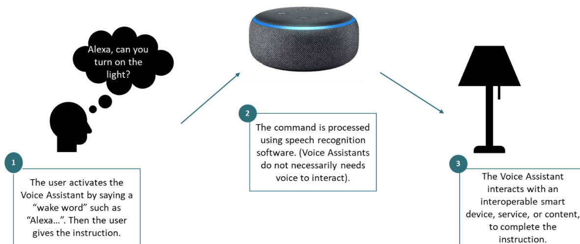
Figure 12 Example of how a Voice Assistant interacts with the user and responds to commands
